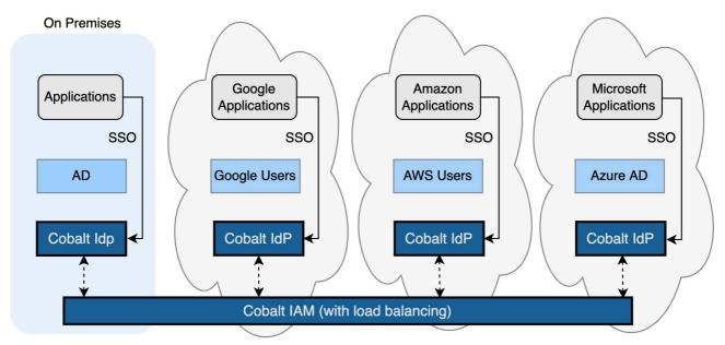
Credentials are synchronized across instances of Cobalt on each cloud platform and on-premises, which allows a user to perform single sign-on from any Cobalt IdP. This ensures that if one platform has an outage, then applications hosted by the remaining platforms are unaffected and remain available to users.
